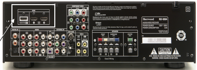
The Sherwood RD-6504 is an HDMI Repeater. It takes in the HDMI signal, processes the audio and sends the video on to the TV.
